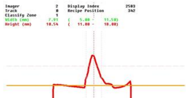
Figure 1b: Bead height failed by GlassMaster due to material expiration
