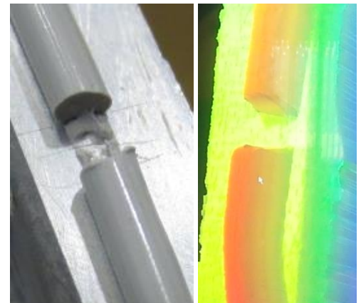
Missing a chunk of bead
