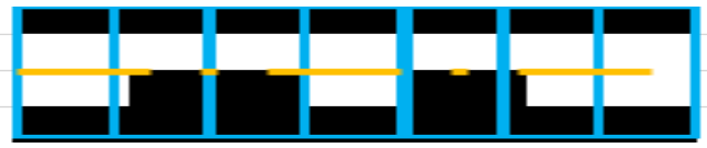
Shiny Oil Pan makes Sealant Bead (white in picture above) “look” thin on 2D vision — False NG
