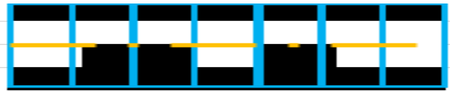
Shiny Oil Pan makes Sealant Bead (white in picture above) “look” thin on 2D vision — False NG
